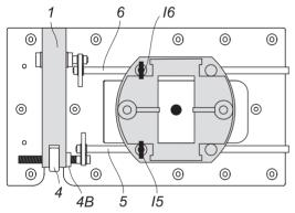
**Tip:** Positioning the router base Wing Bolts towards the bridge end of the CRB7 will increase micro adjuster accuracy.
