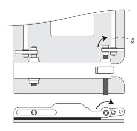
Flip cranked adjuster rod (5) to its outer position.
