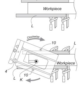
Check that the mortise pillars can complete the mortise without running off the end of the battens.
