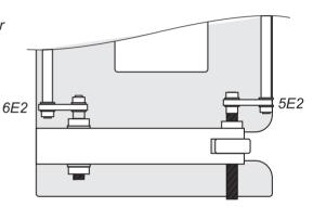
For further adjustment fit the rods in the other crank plate drillings (5E2 & 6E2).
