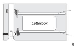
The CRB7 is fitted with 5/16" (8mm) diameter guide rods (5 & 6).
