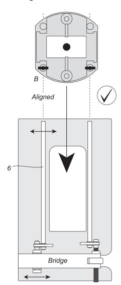
Align fixed rod (6) with the router base rod drilling (B), so that both rods are aligned.
