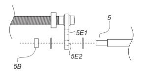
Loosen the M5 nut (5B) using a 5/16" spanner.
