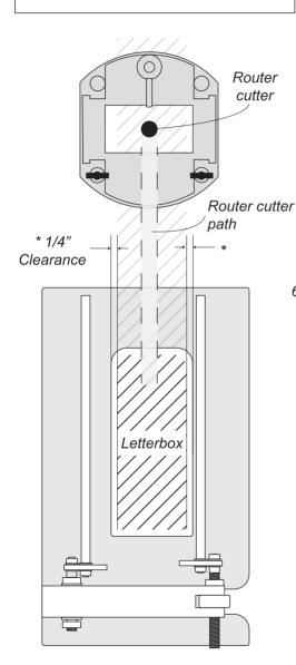
Check that the router cutter will safely align within the letterbox cross hatch area.
