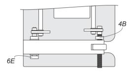
Using 1 x 1/2" (13mm) spanner, slightly loosen fixed rod nut (6E) and micro adjuster nut (4B).
