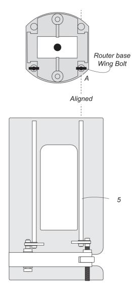
Position the router in front of the CRB7. Align the router base rod drilling (A) with Adjuster Rod (5).
