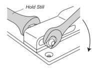
Using 2 x 1/2" (13mm) open ended spanners, tighten both fixed rod nuts.
