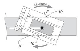
When cutting the mortise, ensure an even pressure is maintained between the mortise pillars and workpiece.
