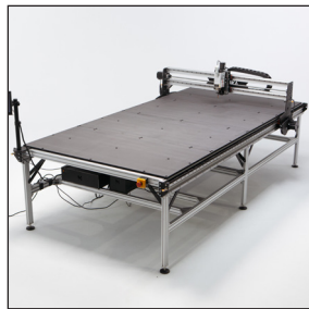
1300x2700mm working area to mill wood, aluminum, plastic and fiberboards
