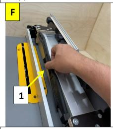
The push stick (1) can be be reinserted. Once all screws have been firmly tightend, the fence is ready for operation.
