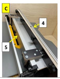
Set the router fence (4) as follows shown on the parallel fence of the saw (5)
