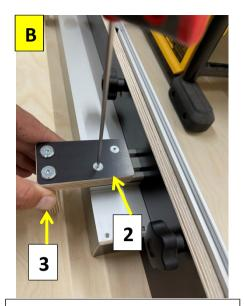
Loosen the screws of the Holding brackets (2) and the clamping brackets (3)
