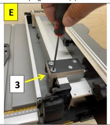
Tighten the screws of the Tighten the clamping brackets (3)
