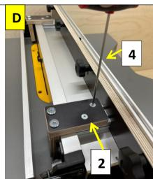
Press the router fence (4) and push the holding blocks (2) against the parallel fence. Tighten the screws of the holding brackets (2) firmly on
