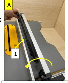
Remove the push stick (1) and fold the parallel depth stop to the saw side
